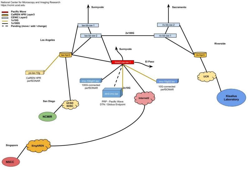
NOTE: this diagram represents a subset of sites, devices, and connections
