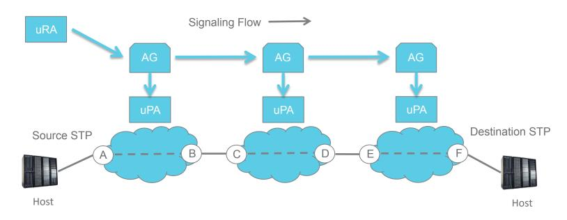
Every NSA associated with network resources must be an Aggregator capable of propagating a reservation request to the local uPA component and at most one adjacent (child) NSA associated with the next connection segment in the data path.
