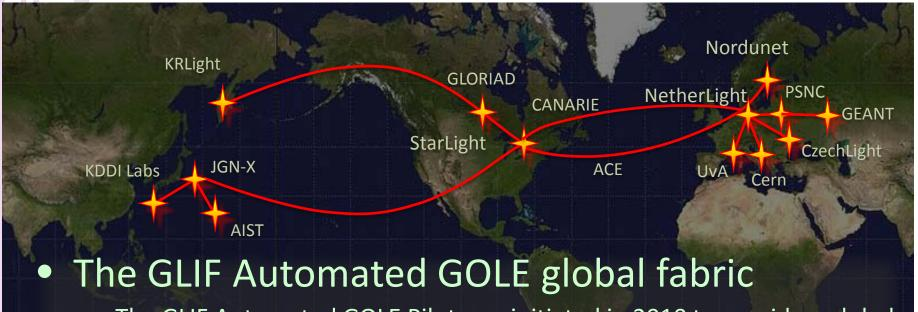
The GLIF Automated GOLE Pilot was initiated in 2010 to provide a global fabric of Open Lightpath Exchanges for the express purpose of maturing the dynamic provisioning software, demonstrating the value of GOLEs to emerging network service models, and to develop a set of BCP for these
