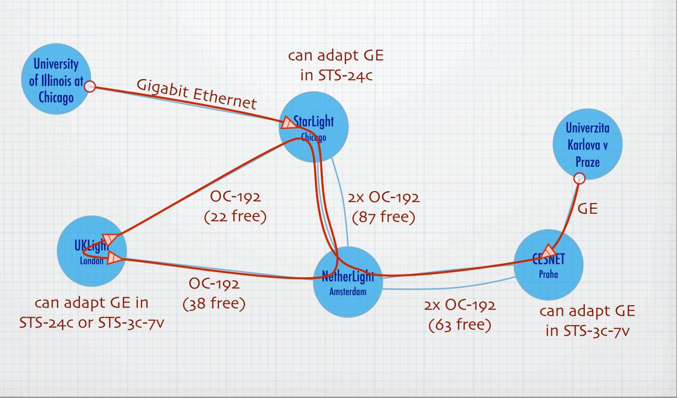
This is the shortest path through this network. You can not just consider one layer in this example: Quebec and Amsterdam do not even know about SDH. NetherLight does not understand Ethernet. Adaptations are important. We need a new "Dijkstra".
