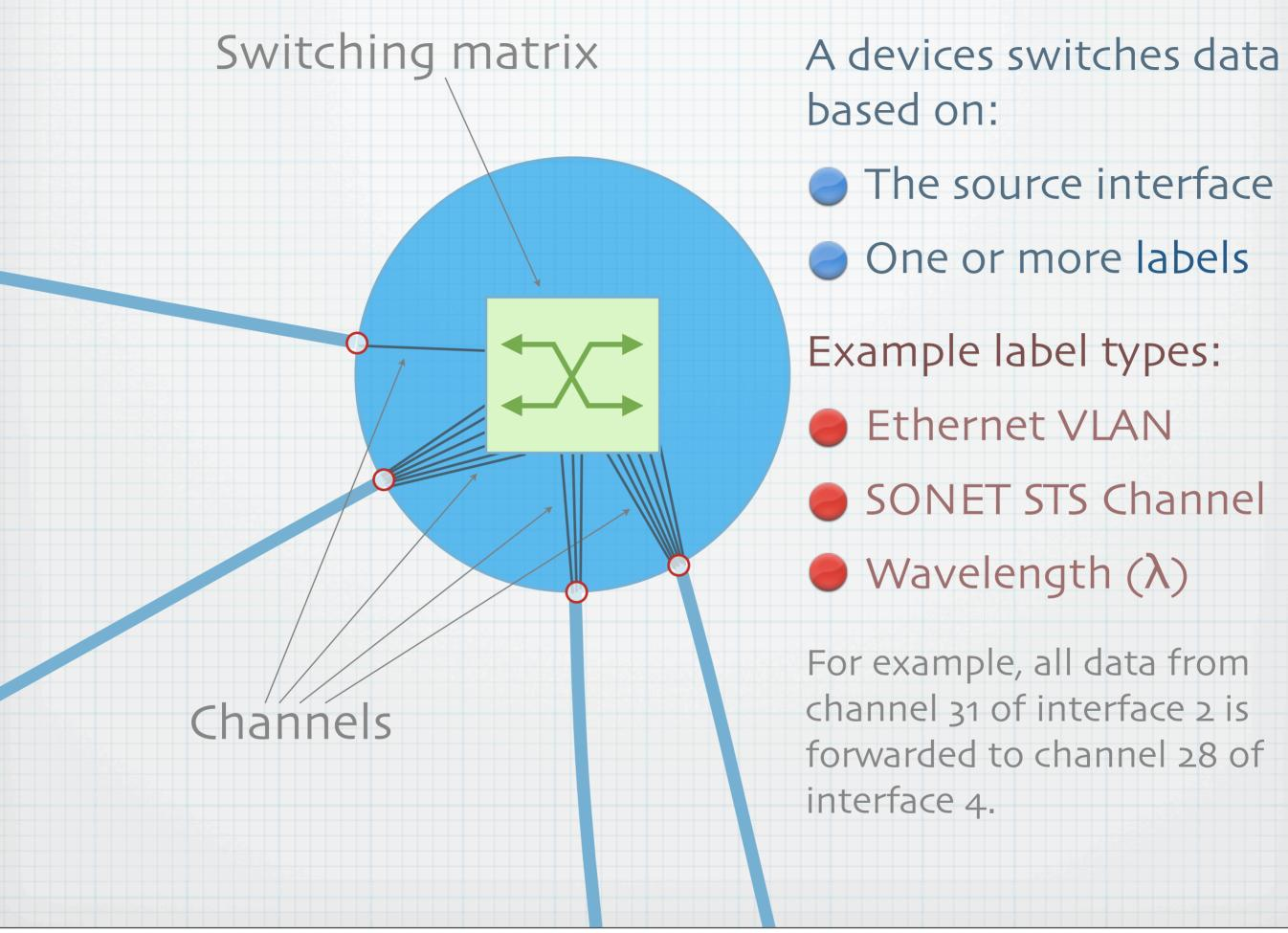
Core of a device is a switching matrix. Typically, every connected link is split (demuxed) into multiple channels, each of which is connected to the switching matrix. Any property that is used to make a switching decision is a label type. GMPLS concept.
