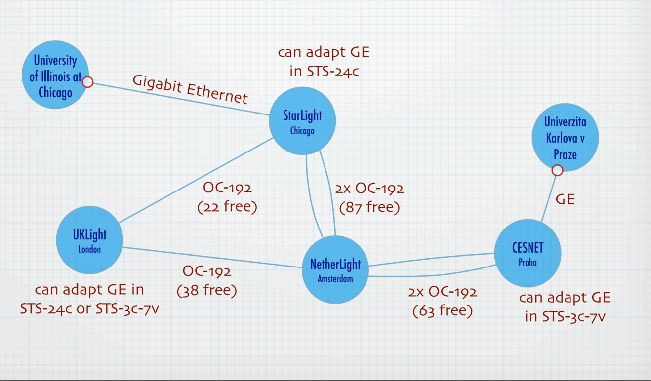
This is our network. It's an example based on a practical problem in the GLIF about 2004. Hybrid: different technologies/layers. Different adaptations between layers. Not all available. Question for the network engineers in the audience: please find the shortest working path from University of Illinois at Chicago to Charles University in Prague.
