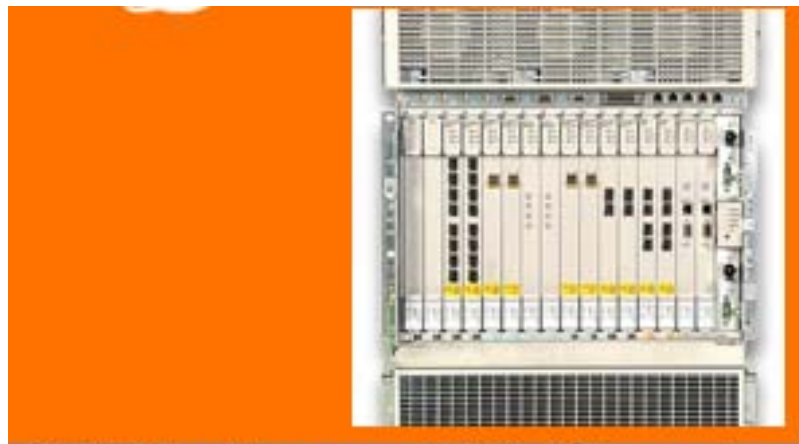
At iGrid, Nortel demonstrated 256-bit AES encryption at 10 Gbps line speeds -- integrated into a standard Nortel Optical Multiservice Edge (OME) 6500 switch.
